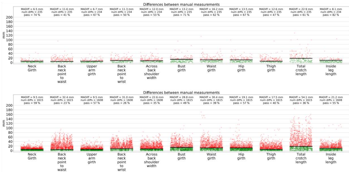
Fig. 2. Differences between manual measurements. The structure is the same as Fig. 1. The top plot shows intra-measurer precision (differences between measurements by the same measurer). For 4 measurers each measuring twice we get 4 differences per scan subject (~240 differences). The bottom plot shows all differences (intra and inter measurer). For 8 measurements per scan subject we get ~1680 differences ((8 choose 2) * 60). That the plots contain a little less data is indicative of missing data or the effect of outlier removal.
