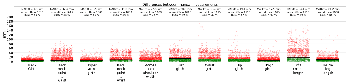
Fig. 2. Differences between manual measurements. The structure is the same as Fig. 1. The top plot shows intra-measurer precision (differences between measurements by the same measurer). For 4 measurers each measuring twice we get 4 differences per scan subject (~240 differences). The bottom plot shows all differences (intra and inter measurer). For 8 measurements per scan subject we get ~1680 differences ((8 choose 2) * 60). That the plots contain a little less data is indicative of missing data or the effect of outlier removal.
